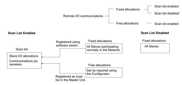
**Note** The scan lists created with the Configurator will be required again for registration in the Master Unit if the Master Unit is ever set to disable the scan list or if the Master Unit is replaced. Be sure to save any scan lists created with the Configurator as network files or master parameter files.
